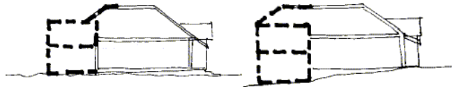
Comment : Generally this type of addition is only successful when the ground slopes away from the front of the property or where the floor to ceiling height is reduced from the original.
